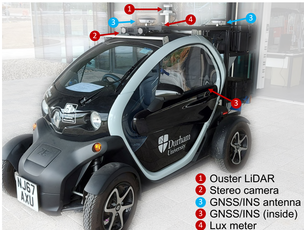
Figure 3.2: Test vehicle (Renault Twizy): equipped with a long-range stereo camera, a LiDAR, a lux meter and a combined GNSS/INS inertial navigation system.
