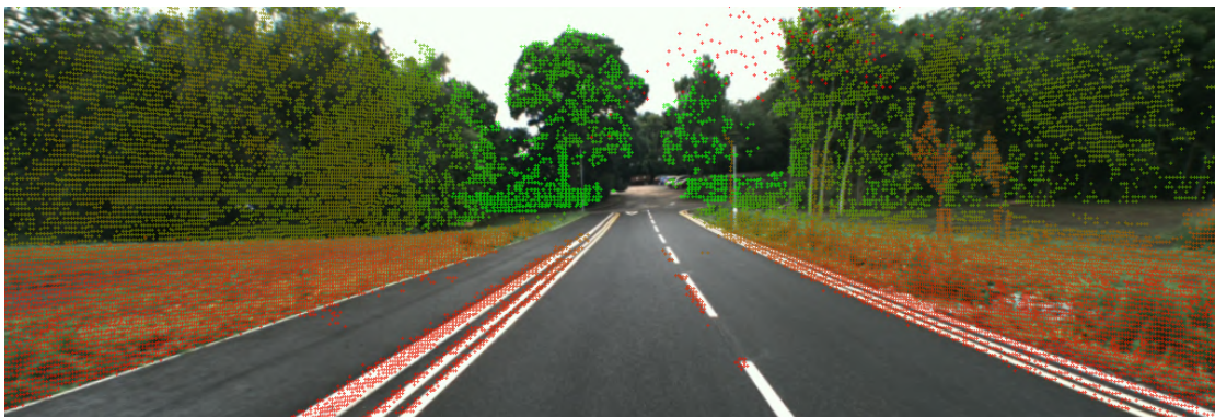
Figure 3.8: Illustrative LiDAR 3D point cloud overlay onto the right stereo image (color) using the calibration obtained.
