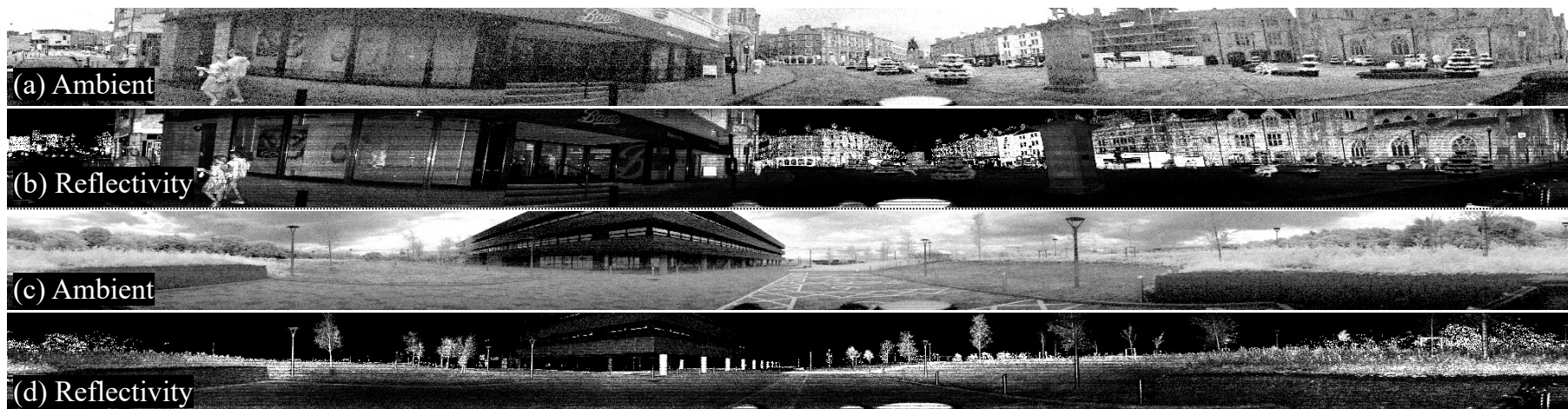
Figure 3.6: Example of ambient (near infrared) and reflectivity panoramic images in real time, all without a camera.
