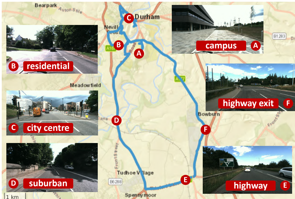
Figure 3.4: The route (blue curves) used for dataset collection showing a variety of driving environments.
